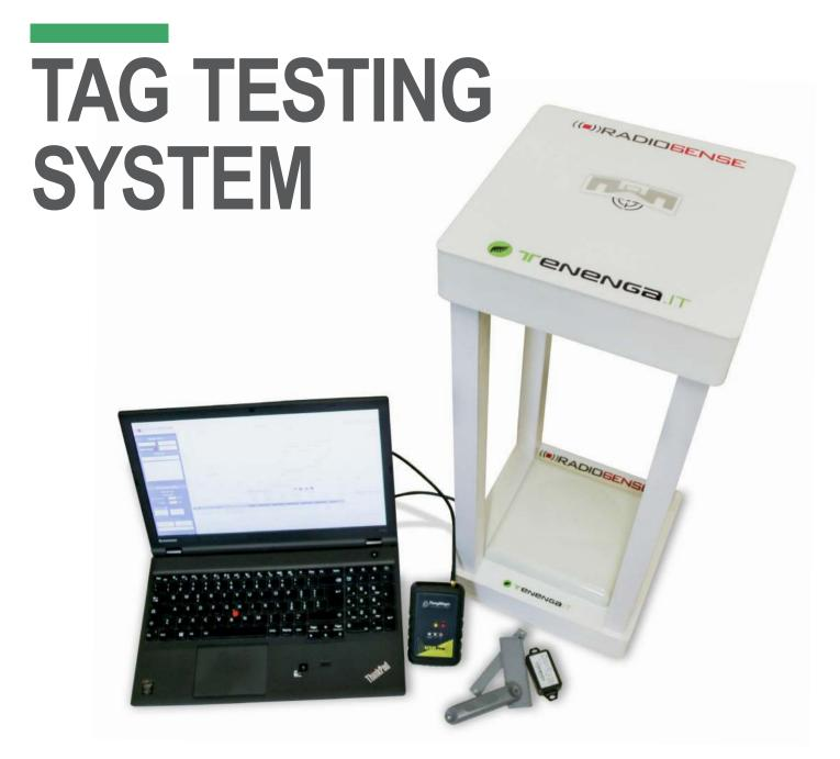
Tag Testing System is a complete, portable and inexpensive kit that allows you to evaluate in real time the functionality and the performance of passive UHF RFID tags.
